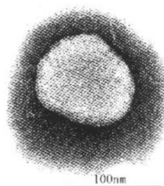
Figure 4 TEM image of SiO 2 /PU nanocomposite with the ratio of 2 : 10 by weight between TEOS and PU.
